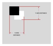
Note: It is important to remember the orientation the part was printed in, as this affects the direction the part will be adjusted in.
