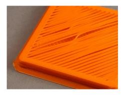
2. Too little extrusion: Inconsistent material extrusion. Layers and rows of extruded material can be skipped and produce an undesirable top layer finish.
