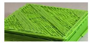
3. Sufficient top layers & extrusion: Top surface will be flat and smooth. No gaps, bulges, or holes in the top surface of part.
