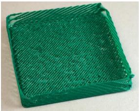
2. The extruder is moving too quickly. The beads are not bonded together and appear stretched and messy. Possibly missing some material or material has fallen into the middle of the box.
