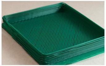
3. The filament feed and extruder speed are correct. The feed rate of the material and extrusion multiplier match the speed of the machine. The material bonds well together.
