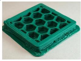
2. Blobs in the corners of the part: Improper settings for extruder movements and retracts can cause globs and zits on the outer walls of the material.
