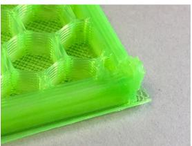
3. Good, connected infill patterns: Good material flow speeds and retract settings. Adjust retract settings to control material flow between layers. Adjusted feed rate and extrusion multiplier to control material flow while extruding.
