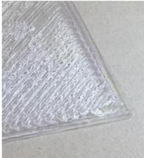
2. Nozzle is too high. The chip may fall apart after removing from the print bed. Diagonal infill lines will not be joined together, and will pull apart like strings. Because the nozzle is too high, the bead of material is not flattening as it should.
