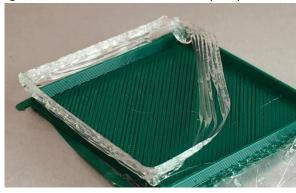
2. Is the extrusion consistent? Over extrusion or under extrusion o the material may occur. Slow feed rates or incorrect nozzle settings may cause globs and messy prints.
